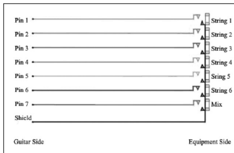
Fig. 11.4 13-pin breakout box schematic
