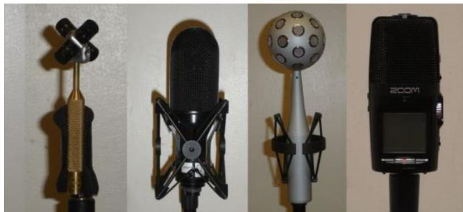
**Figure 8** - Various Soundfield Microphones (from left to right): Core Sound TetraMic, Soundfield MKV, MH Acoustics Eigenmike, and Zoom H2n [4]
